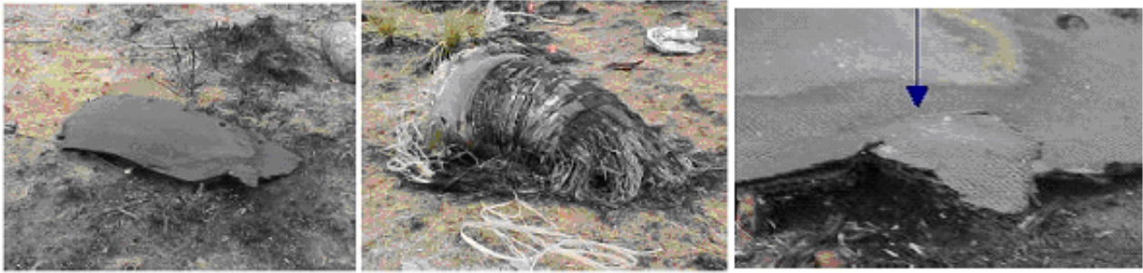
Figure A4.4. Typical Crash Site Damaged Composite Material
